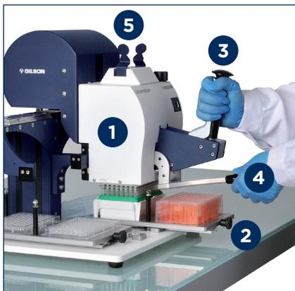
The device is now ready to pipette liquid.
