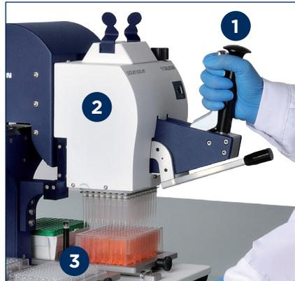
To simplify this operation, the height adjuster **3** can be set by turning the upper screw so that the pipetting head may only be moved down to a position slightly above the bottom.
