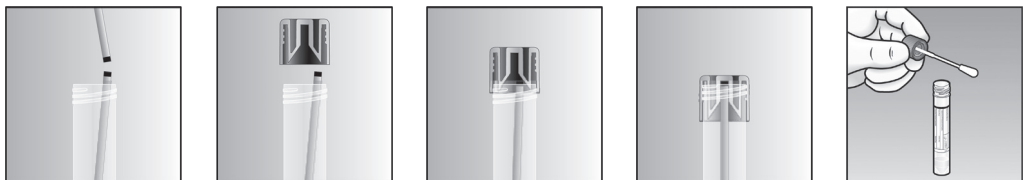
Fig 3. Capture of broken swab applicator stick by FecalSwab™ tube cap
