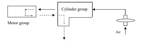
After the pipette is installed properly, pressing the control buttons (Aspirating Button & Dispensing Button) would start the motor group to generate a vacuum in the pipette. Then the air/liquid would follow the vacuum into the pipette. The sucking speed can be adjusted by pressing the blue buttons marked with +or-.
