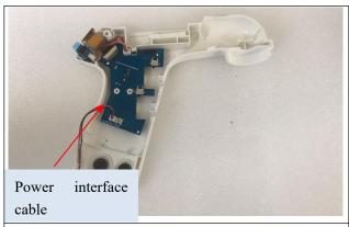
9-replace master control board (circuit assembly) step1:
