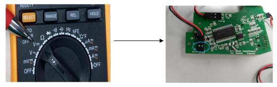
Please turn the multimeter to DC scale, then connect the two pens to the two ends of the motor as shown in the picture.
