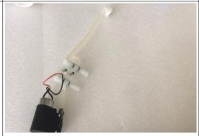
8-replace the pump and cylinder group - step2: Taking out the pump and cylinder group,then dismantle them separately.
