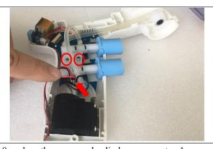
8-replace the pump and cylinder group - step 1:
