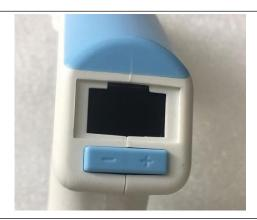
3-Open the LED display with a blade, and take it down. (gluing the LED display when re-installation).
