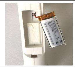
5-Take out the battery,unplugging the cable terminal, please note the polarity.
