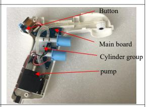
7-Seperating the shell , we can see the internal components.
