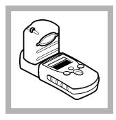
**5.** Install the instrument cap over the cell holder.
