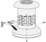
9.2.2. Carefully ease the base away from the main body. The fuses are connected via the connection block secured to the base.
