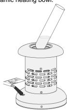
7.2.6. Crucible heating may be achieved by removing the cowl. (It is recommended that protective gloves should be worn when removing the cowl). The cowl is removed by rotating in the direction indicated in the illustration below.
