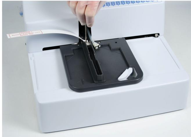
**Figure 9–27.** Fastening the transport lock
