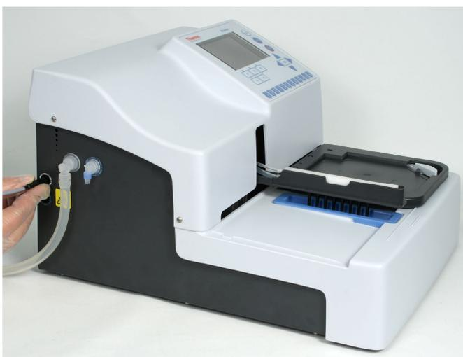
**Figure 3-17.** Connecting the liquid sensor cable
