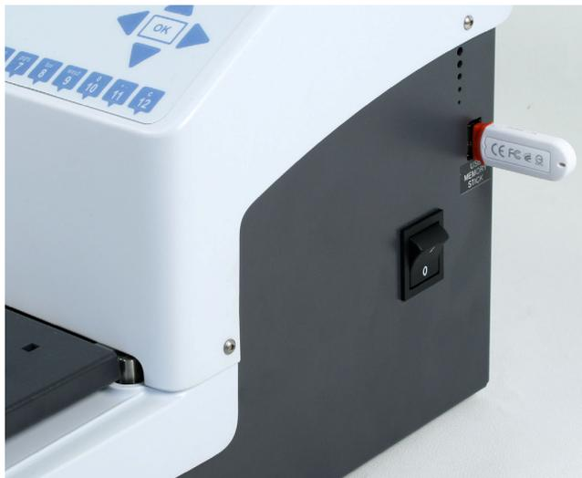
**Figure 6–24.** USB memory stick inserted
