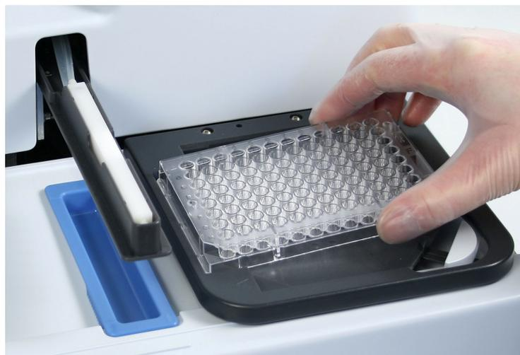
**Figure 4–21.** Inserting the microplate
