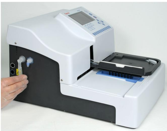
**Figure 3-16.** Connecting the liquid container tubing
