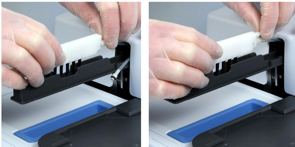
**Figure 3–11.** Fitting the wash head to the tubing
