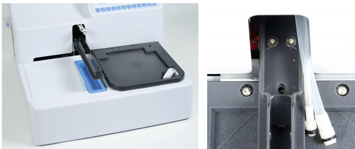
**Figure 9–26.** Aligning the plate carrier and wash head arm
