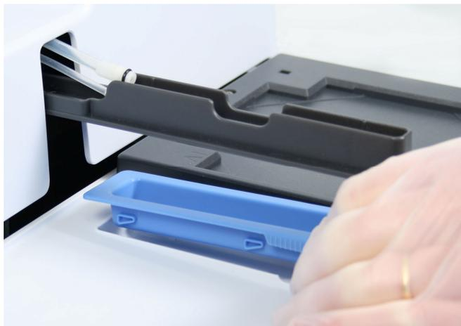
**Figure 3–9.** Removing the priming vessel
