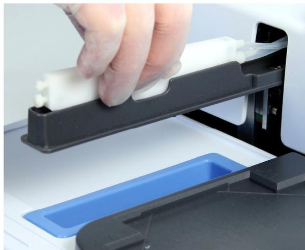
**Figure 3–12.** Fitting the 1 x 8 wash head onto the wash arm
