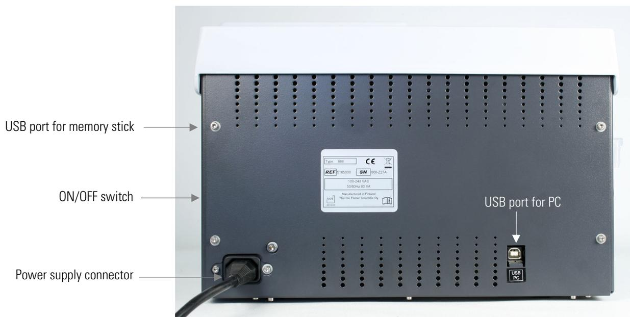
**Figure 3–20.** Connecting the power supply cable
