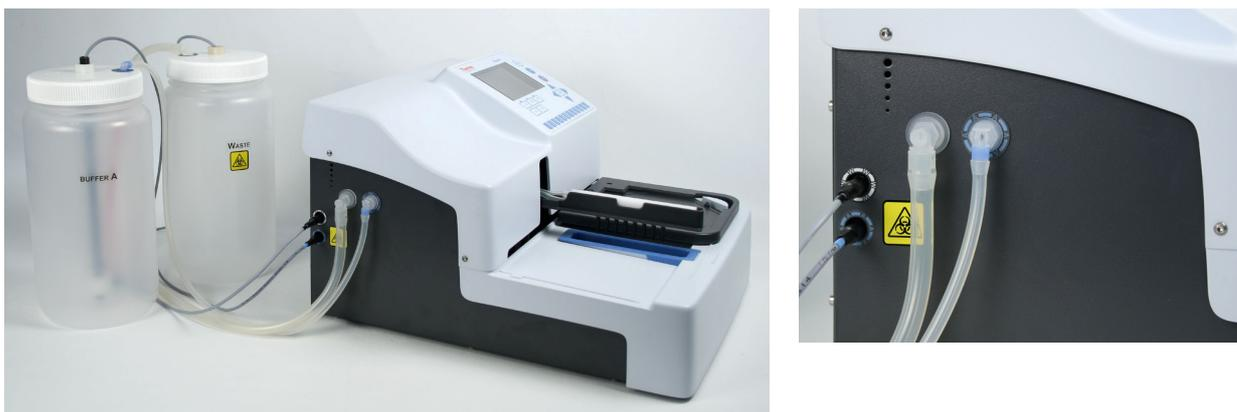
**Figure 3–18.** Liquid containers connected to the instrument
