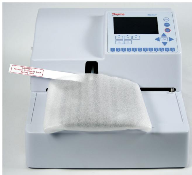
**Figure 9–28.** Transport lock and tag fitted
